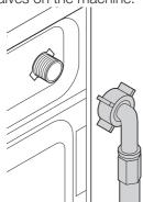
In order to prevent water leakage that may occur at the connection points, there are rubber seals (4 seals for the models with double water inlet and 2 seals for other models) attached to the hoses. These seals should be used at the tap and machine connection ends of the hoses. The plain end of the hose fitted with a filter must be attached to the tap and the elbowed end must be attached to the machine. Tighten the nuts of the hose well by hand; never use wrenches to tighten the nuts.
